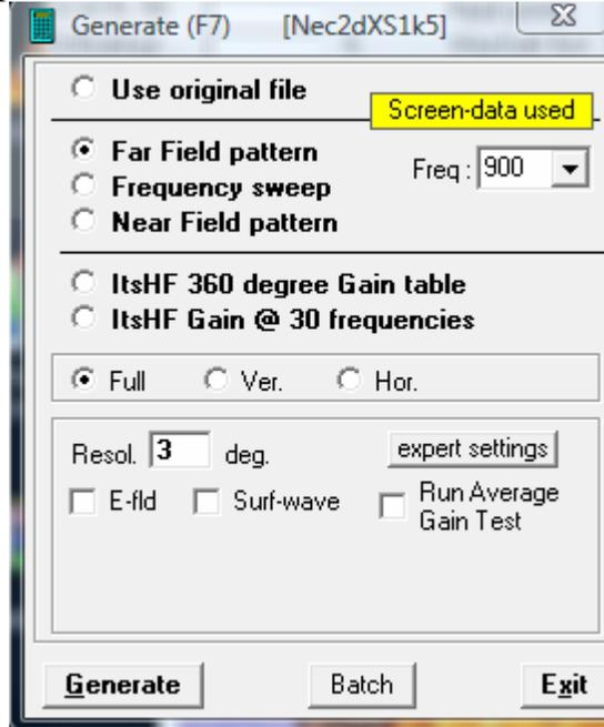
*Far Field pattern:* Used for calculating Far field antenna parameter
